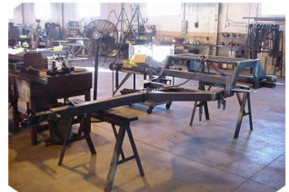
Custom Fabricated Trailer Frames for Pavement Friction Test Trailer
